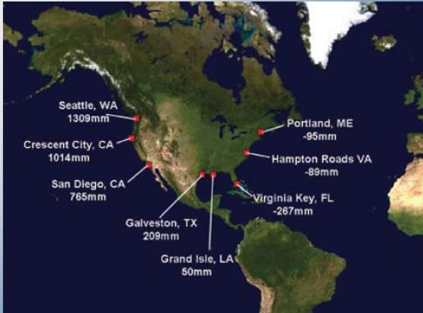
Figure 3. Elevation difference between LMSL (1983-1999 NTDE) and NAVD 88. [Note: The LMSL for Grand Isle, Louisiana is based on the 2001-2006 Modified Tidal Datum Epoch and an updated NAVD 88 epoch 2006.81 specific to the Louisiana region.]
