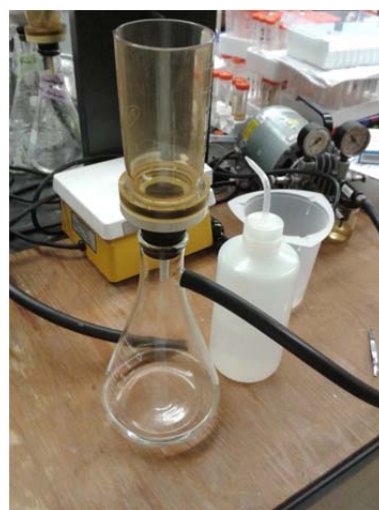
Figure 3: Filtration setup used in TSS
