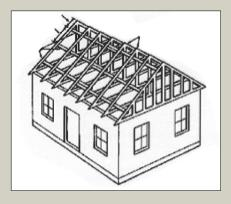
**Figure 4-6.** The trusses are built with a peak at the ridge line of the house. The trusses at the end of the house form an A-shaped pattern known as a gable end. During a hurricane, the gable end is subject to great forces from the wind and is likely to tip over, collapsing the other trusses in a domino fashion. Source: FEMA's *Against the Wind* brochure 247.
