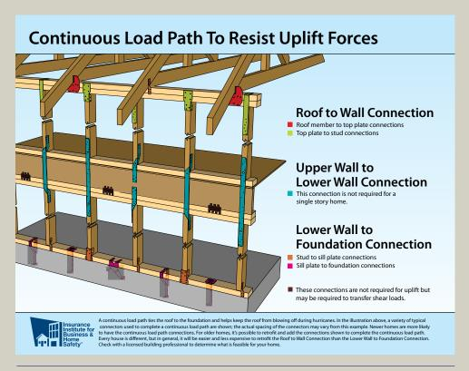
**Figure 4-4:** Continuous load path connection ties: the roof to wall, usually with hurricane clips and plate ties; the wall of a higher story to the wall of a lower story with straps; and the wall to the foundation with plate ties and anchors. Continuous load path connection ties should be in all new houses. Older homes usually will not have these features. In many cases, retrofit can easily be done for certain portions. Source: Simpson Strong-Tie.
