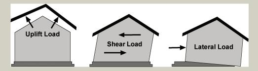
**Figure 4.3.** Strong winds create three types of force on your house. The uplift load occurs when wind pressure pushes a roof up from beneath or when wind flows over the house and pulls the roof up. The shear load occurs when horizontal wind pressure causes the walls of the house to tilt. The lateral load occurs when wind pressure on the walls causes the house to overturn or slide off the foundation. Source: Louisiana Sea Grant.
