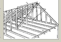
Hip-style roofs do not need as much bracing, as they are aerodynamically superior and have bracing built into the design of the structure. While gable-end roofs have a flat end that is A-shaped, hip-style roofs are similar to a pyramid and have the tops of all four sides of the roof sloping toward the center of the roof.
