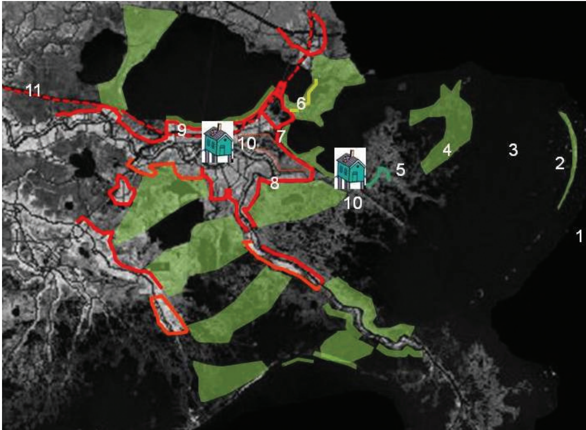
Figure 3-2. Example distribution of lines of defense in southeast Louisiana: (1) Gulf of Mexico shelf, (2) barrier islands, (3) sounds, (4) marsh land bridges, (5) natural ridges, (6) highway foundations, (7) flood gates, (8) levees, (9) pumping stations, (10) elevated homes and buildings within levees and outside levees and (11) evacuation routes (From J.A. Lopez. 2006. The Multiple Lines of Defense Strategy to Sustain Coastal Louisiana . Lake Pontchartrain Basin Foundation, available at http://www.saveourlake.org ).
