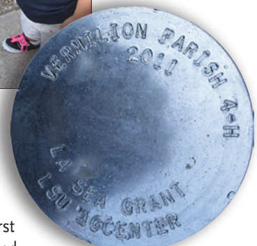
Mark Shirley and students set an elevation benchmark in concrete.
