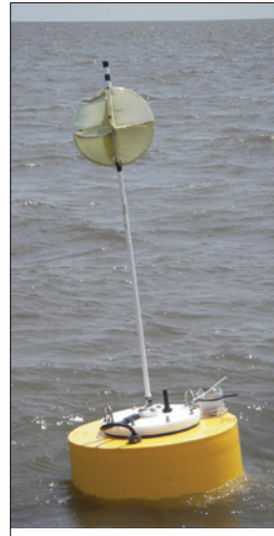
This is one of a series of three buoys that relay information from fish transmitters.
