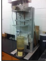
Lick shaker apparatus at UNO
