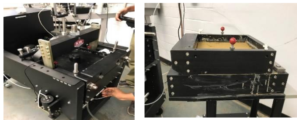
Figure 2 (left) The large-scale direct shear test machine, (right) the 12 in ×12 in shear box after a test was completed
