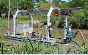
Theoretically, the dredge can pump up to 70 percent solids at a rate of 20 cubic yards per hour through a 4-inch hose. This converts to filling a one-acre area with a one-foot depth of dredged material in 75 hours.
