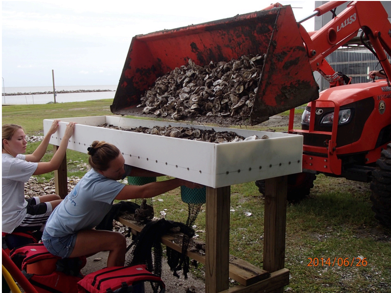
Figure 9. Shell bags being filled at a table designed to aid in filling. Bags are slipped over the PVC pipe affixed to the table; cultch is then loaded onto the top of the table and pushed into the openings filling the bags.
